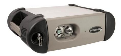
A rugged and reliable post-dispersive near-infrared spectrometer designed for the industrial, manufacturing, laboratory, and field environments, providing research-grade materials measurement information, where and when you most need it.
