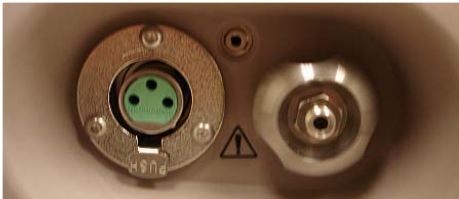
Figure 2-8 Enhanced view of the front panel with the fiber optic cable connector, port for remote trigger, and accessory power port for probe.
