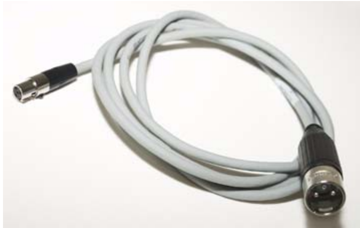
Figure 2-9 Cable used from the TerraSpec spectrometer accessory power port to the Contact Probe, MugLite, or other authorized ASD accessory.
