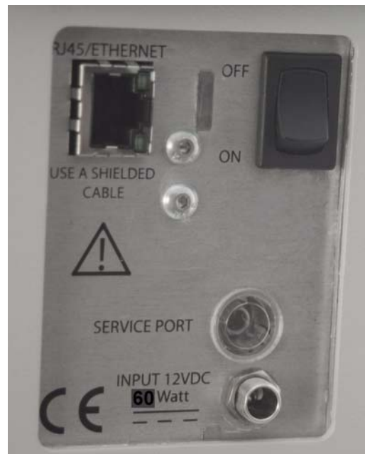
Figure 2-6 TerraSpec spectrometer back panel showing Ethernet connection, power switch, and power input jack.
