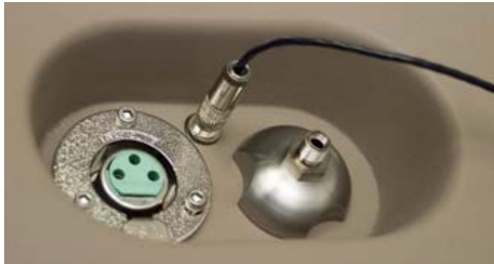
Figure 2-11 External trigger cable plugged into the TerraSpec spectrometer.
