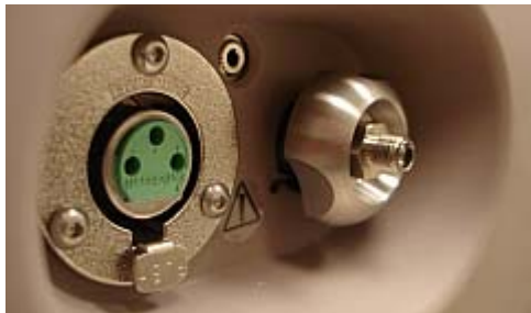
Figure 4-2 View of the fiberoptic bundle matcher and the fiberoptic port.
