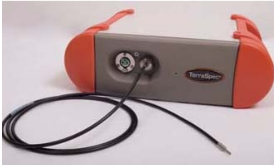
Figure 2-2 TerraSpec spectrometer front-view showing fiber connection and power output.
